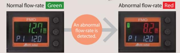
\* In these examples, the value to determine abnormal flow rates is set at 12.0 L/min.
