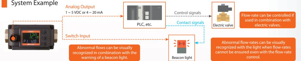
Flow-rate can be controlled if used in combination with electric valves.
